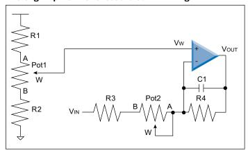
In the following circuit, a resistor ladder is used to create a voltage window where Pot1 is used to trim the desired offset for the non-inverting amplifier. A second potentiometer is used in a rheostat mode to control the gain of the amplifier. The step resistance of Pot2 relative to resistor R3 determines if the gain trimming is a fine adjustment or a course adjustment. Capacitor C1 is for compensation of the op amp and to inhibit the output from oscillating.
